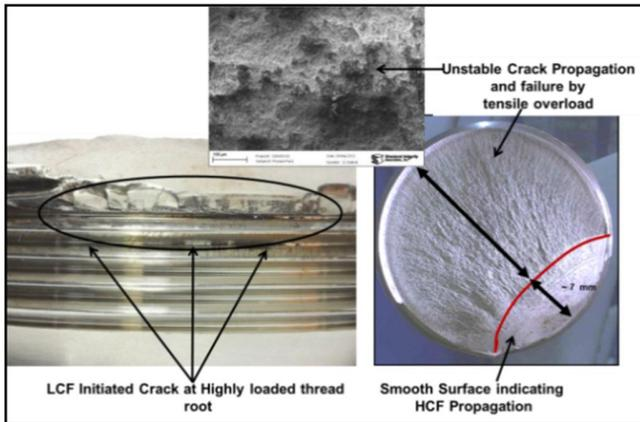
Figure 18: Crack initiation and propagation surface
