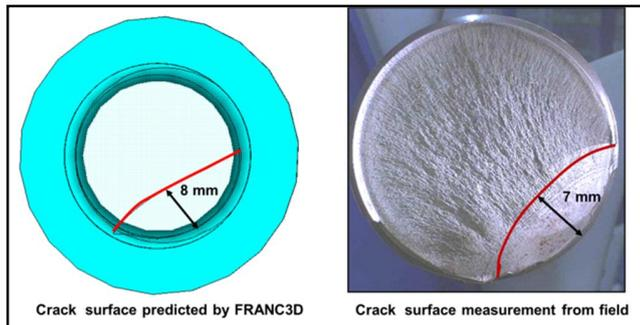
Figure 19: Analytical prediction comparison to field measurement
