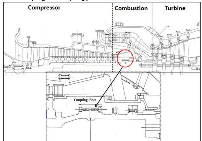
Figure 1: Engine cross section
