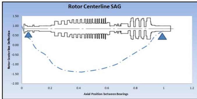
Figure 6: Rotor center line sag (bending mode)
