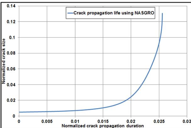
Figure 11: Crack propagation life using NASGRO
