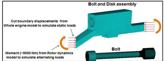
Figure 4: Meshed model with boundary conditions
