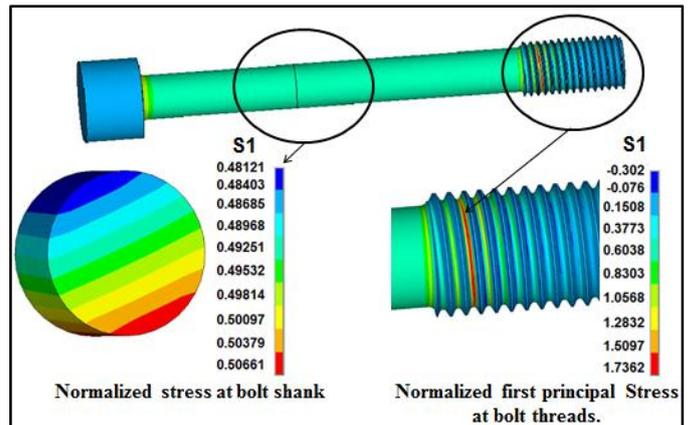
Figure 5: Bolt thread mean stress at baseload operation
