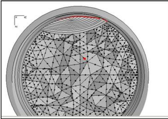
Figure 14: Crack propagation in FRANC3D
