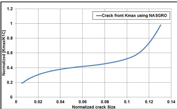
Figure 10: Normalized  $K_{max}$  (vs) crack Size
