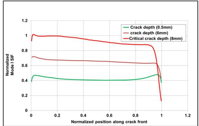
Figure 15: Variation of Mode I SIF along crack front
