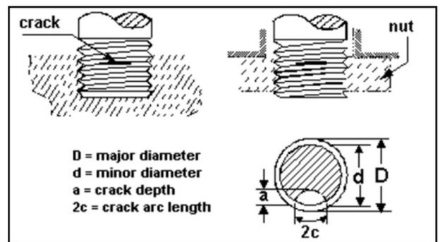
Figure 8: Thread crack set-up using NASGRO
