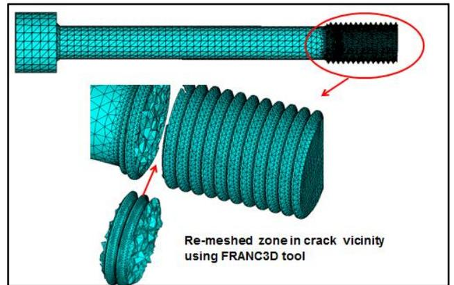
Figure 12: Cracked bolt mesh using FRANC3D
