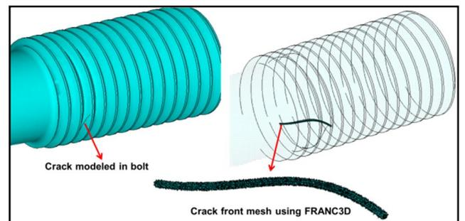
Figure 13: Crack front elements from FRANC3D
