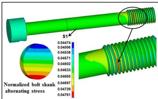
Figure 7: Bolt alternating stress at baseload operation
